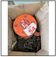
Lot #54 - CHAIN HOIST, MAXON 1 1/2 TON, TYPE MX-HC, LIFT 10 FT ( USED )
