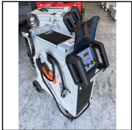
Lot #19 - MIG WELDER, FY-TECH M-PRO MODEL 4250/2E, 250A, 1 PHASE ( NEW DEMO )
