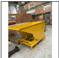
Lot #40 - SERVICE TIPPING BIN WITH FORKLIFT LIFTING POCKETS, 900KG CAPACITY ( NEW SHOP SOILED )
