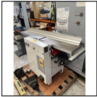
Lot #17 - WOODWORKING JOINTER/PLANER LAZZARI (ITALY) MODEL LFS35 ( WORKING BUT BED SLIGHTLY OUT OF LEVEL )
