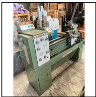
Lot #32 - ENGINEERS LATHE, TRUPRO TPG1340, 330 X 1000, 2HP, 1 PHASE ( USED, EX SCHOOL TRADE-IN )
