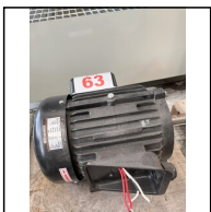
Lot #63 - ELECTRIC MOTOR, 3 HP, 1 PHASE ( SLIGHTLY USED ON A MACHINE ,CHANGED FOR A 3 PHASE MOTOR )
